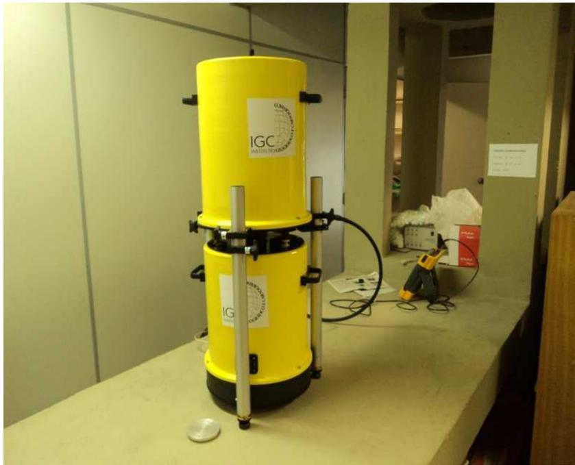
***Figure 8 - Absolute gravity meter A10-32.***
