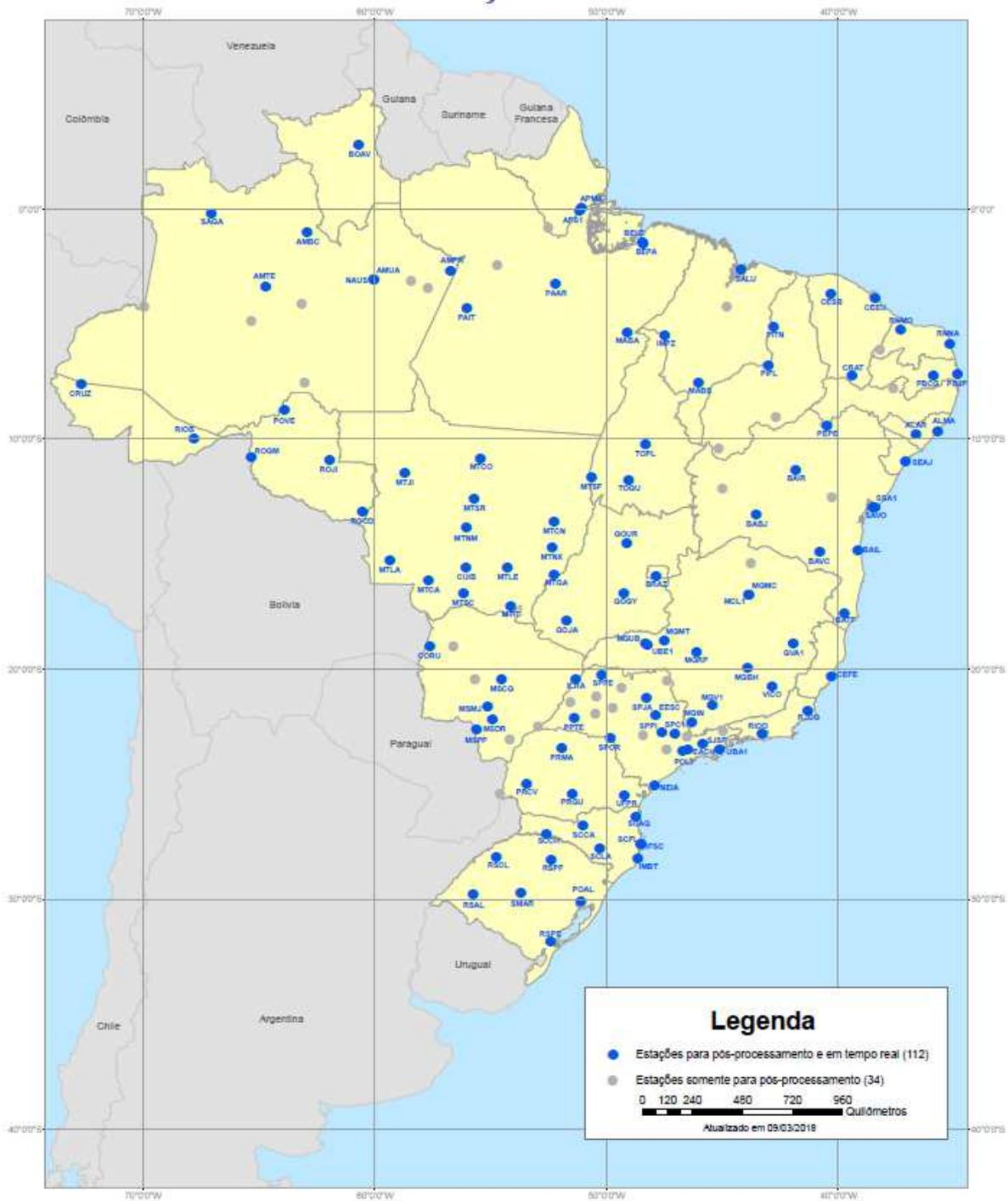
**Figure 6 - The Brazilian Network for Continuous Monitoring of GNSS (RBMC). The current status of RBMC stations. Blue dots representing real-time and post-mission stations, whereas black dots (34) represent post-mission stations.**
