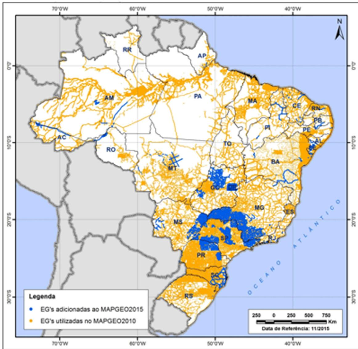
*Figure 2- Status of gravimetric surveys used for MAPGEO2015 geoid model.*
