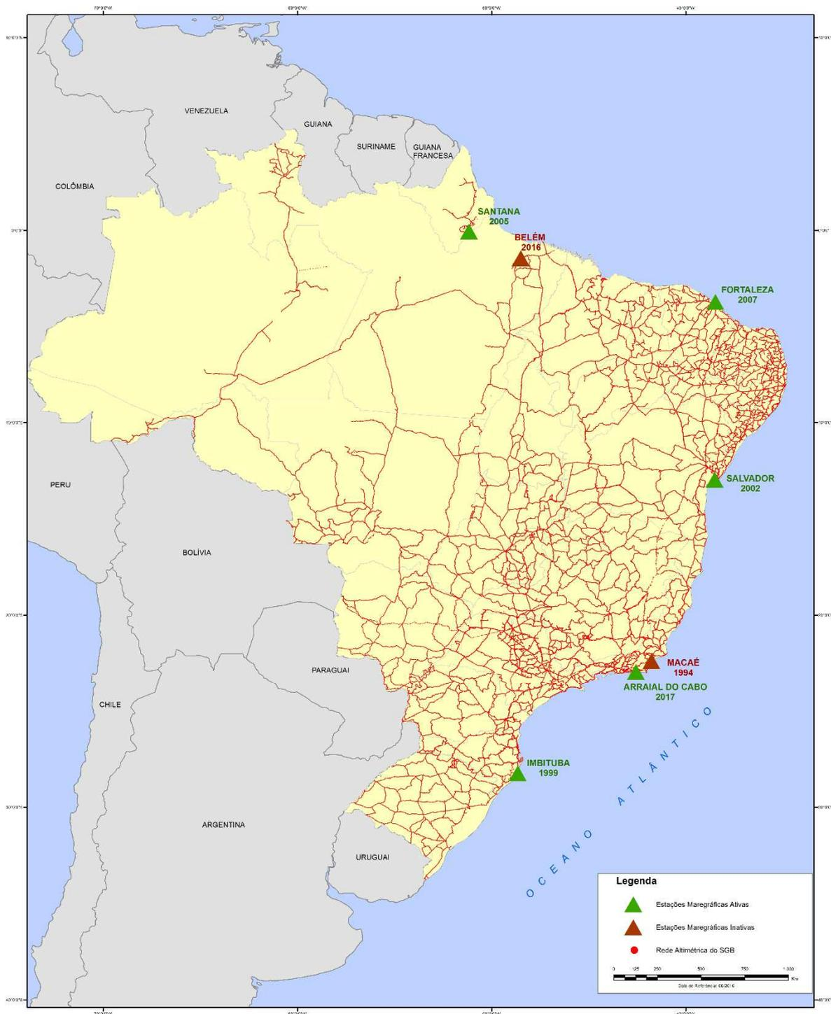
**Figure 1- Brazilian Network of Tide Gauges for Geodesy – RMPG. In red is the spirit levelling network.**
