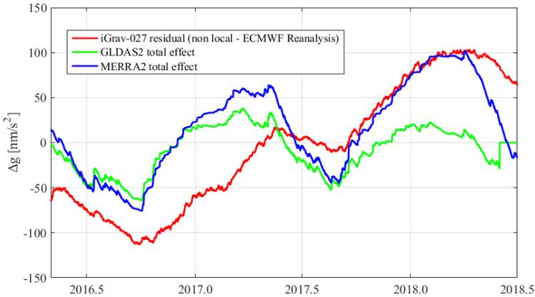
Fig. 14. iGrav-027 residual (red) compared with hydrological loading effect from GLDAS2 (green) and MERRA2 (blue)
