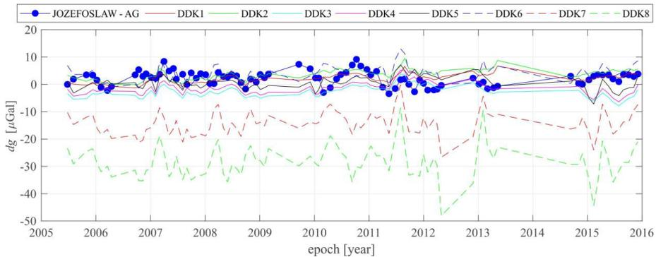
Fig. 20. Differences between variations of absolute gravity determined with the FG5-230 at Jozefoslaw and gravity variations from GRACE-based GGMs provided by CSR
