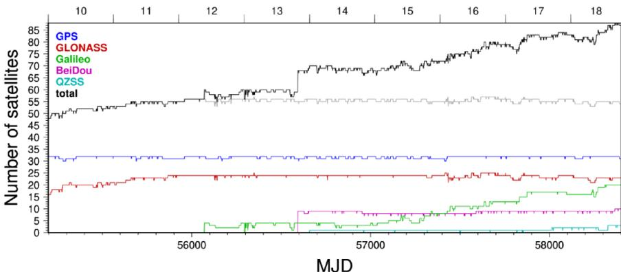
Fig. 7. Number of GNSS satellites: GPS, GLONASS, Galileo, BeiDou, and QZSS included in CODE MGEX solutions in the period 2010.0 and 2018.8, after Dach et al. (2018)
