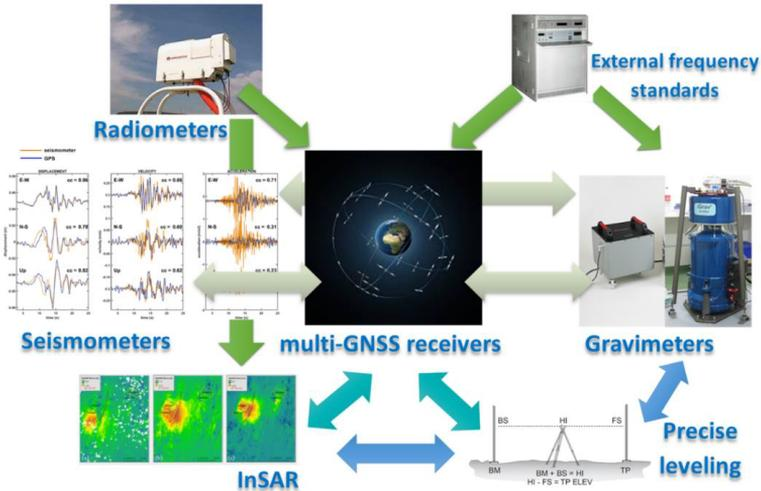
Fig. 14. Co-location of various space geodetic techniques for surface displacements and earthquake monitoring in the framework of GGOS-PL (task 8) in EPOS-PL
