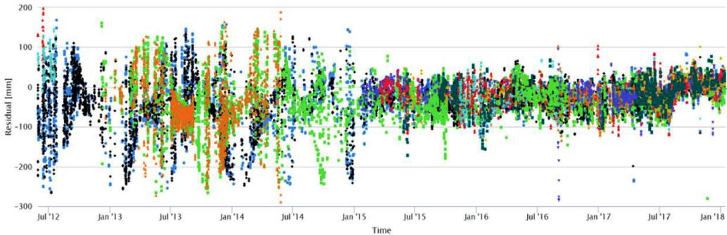
Fig. 8. Evolution of Galileo orbit accuracy as measured by SLR. Figure generated in the GOVUS service (Zajdel et al., 2017)
