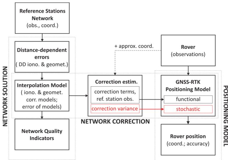
Fig. 1. Network RTK positioning model based on NBSM
