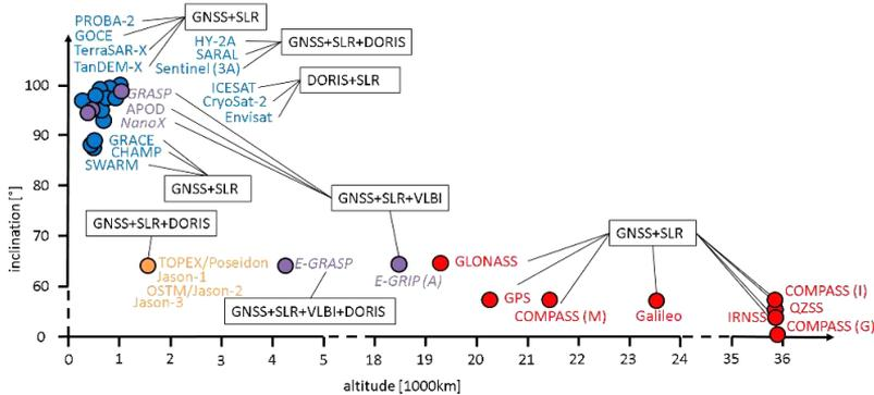
Fig. 3. Available satellites for co-location in space ordered by their altitude and inclination; planned missions are set in italics; after Maennel (2016)
