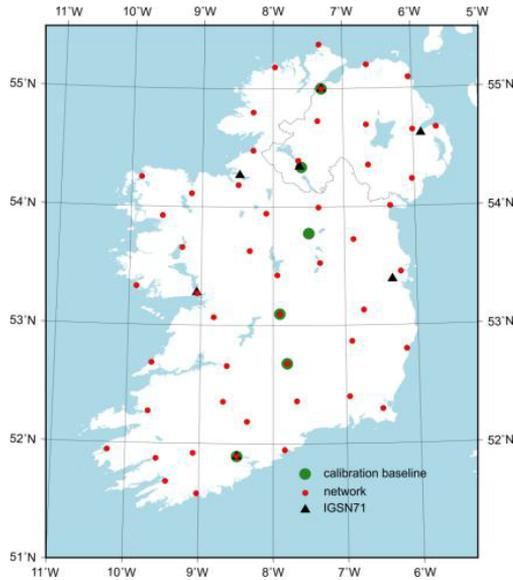
Fig. 6. Design of the Absolute Gravity Network in Ireland
