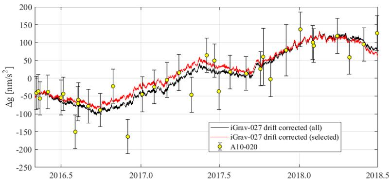
Fig. 13. Combined A10-020 and iGrav-027 records (after drift removal)
