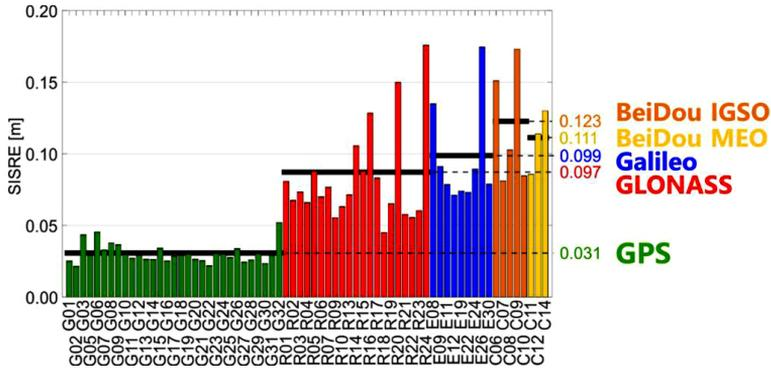
Fig. 9. Signal-in-space ranging errors (SISRE) for CNES multi-GNSS real-time products in 2016, after Kaźmierski et al. (2018b)
