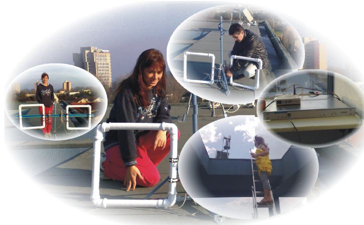
Figure 9: Magnetic VLF and LF antennas installed on the roof of the Dobrudja Observatory
