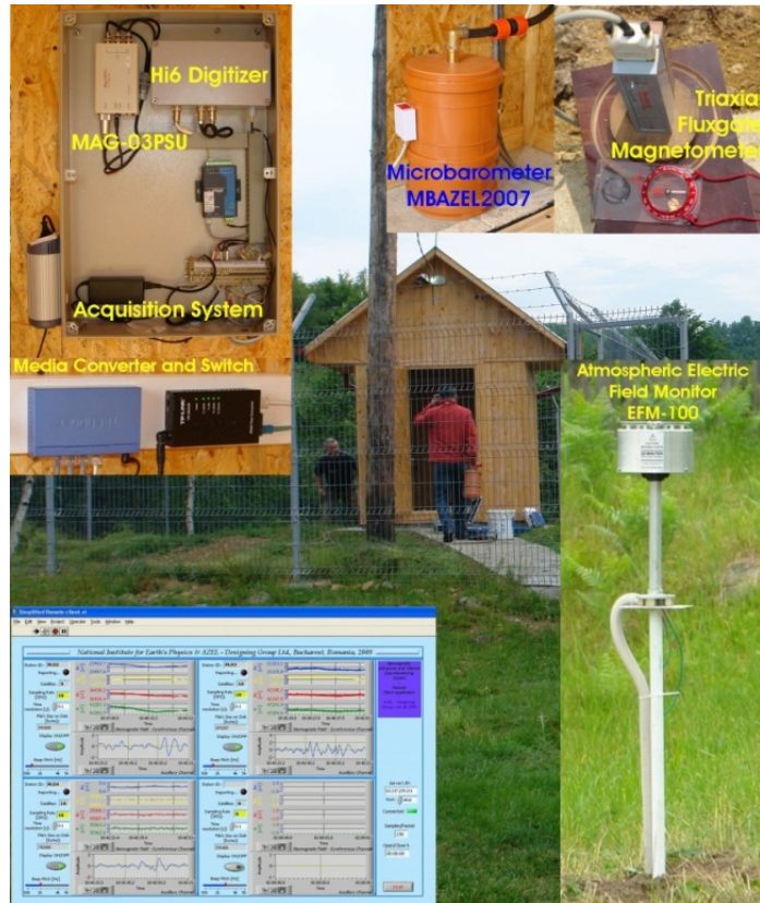
Figure 6: An outer image of PLO3 site and some of the equipments that are involved in the monitoring process: Data Acquisition System, Microbarometer MBAZEL2007, Triaxial Fluxgate Magnetometer MAG-03MS. The Electric Field Monitor EFM-100 is installed at PLO4, in the vicinity of the Weather Station WS-3600.
