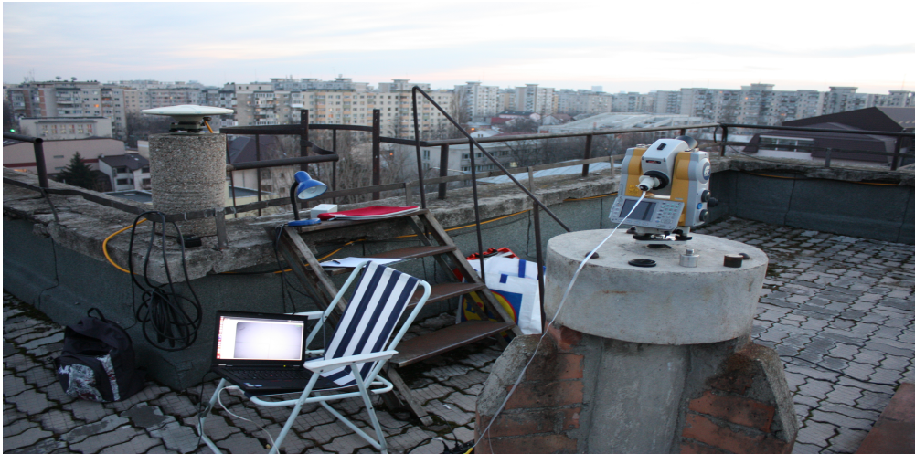
Figure 23: Astro-geodetic observations for vertical deviation determination
