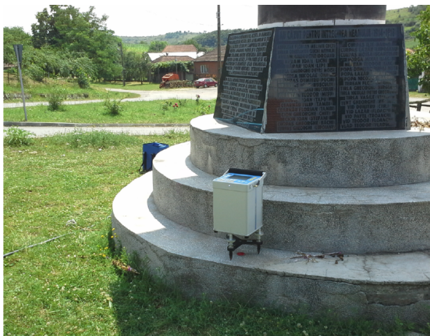
Figure 22: Gravity observations with Scintrex Autograv CG5
