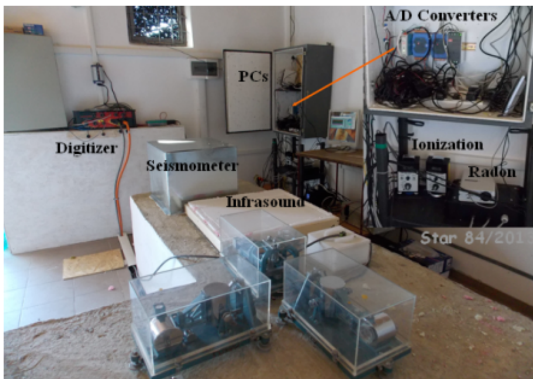
Figure 11: VRI monitoring station
