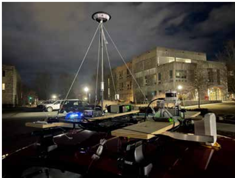
Data acquisition platform installed on a car roof including time synchronized lidar, IMU and GNSS sensors.
