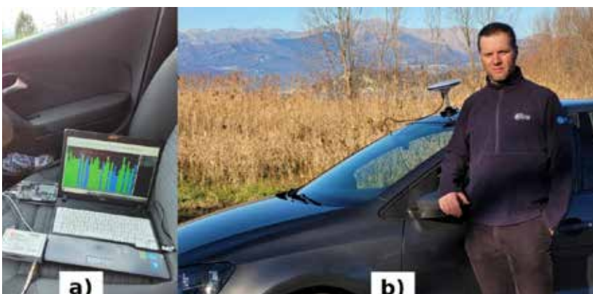
Figure 2: Equipment used for the dynamic tests. a) Internal view of the vehicle with the laptop, reference receiver and front-end adopted for the data collection. b) External view of the vehicle with the multi-frequency antenna mounted on the roof.
