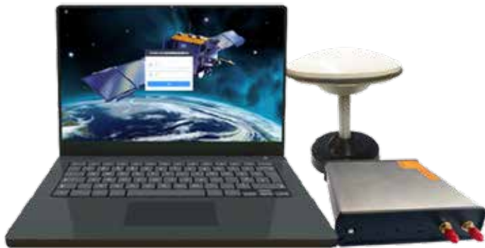
The THUEESDR, the software-defined-radio (SDR) receiver developed by Tsinghua University Electrical Engineering Laboratory. By utilizing the THUEESDR, the developers deployed a CDO-based SQM algorithm toward dual-frequency signals of the four core constellations. Eight metrics are applied, and the optimal code-phase BIN length for BDS B1C/B2a combinations is 0.020 L1-chips or 0.20 L5-chips.
