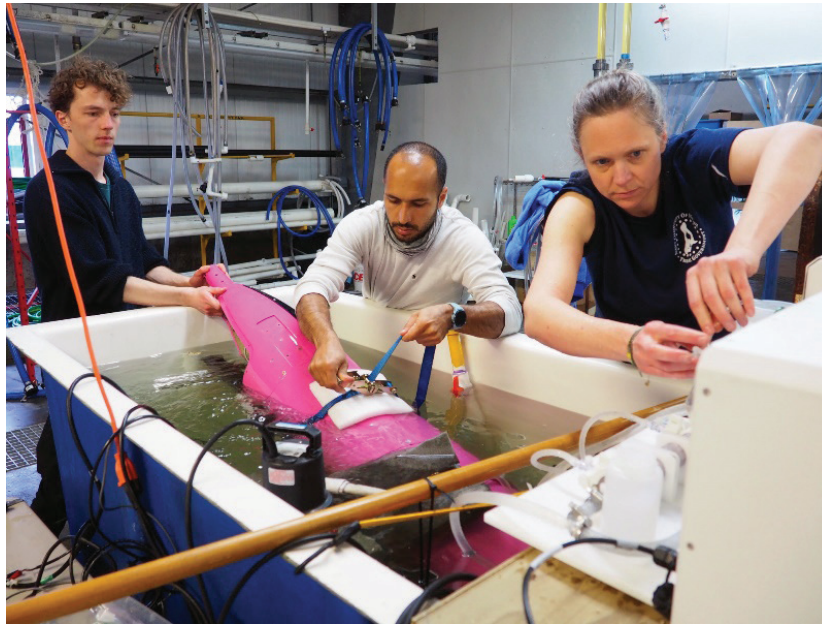
From left, Kemme, Abdi and Hauri compare measurements taken by the Seaglider with lab instruments at the Alutiiq Pride Marine Institute to ensure the accuracy of the data being gathered. Heather McFarland
