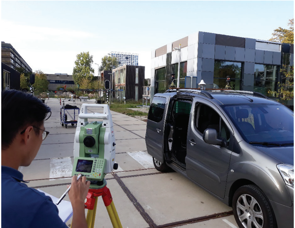
Impression of experiments carried out with a road-vehicle (with the white receiver antenna on top), using the prototype system deployed at The Green Village on TU Delft campus; the self-tracking total station in the front is used to deliver the ground-truth trajectory of the car in this experiment.
