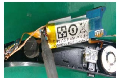
Remove battery wire.
