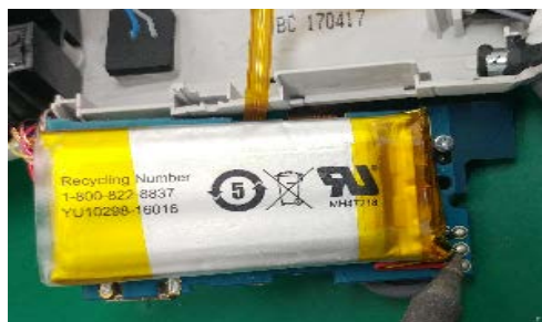
Remove battery wire.
