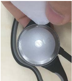
Using a tool, detach Upper case.
