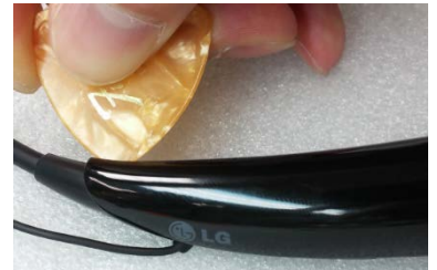
Insert the tool to the edge, and then disassemble from left to right.
