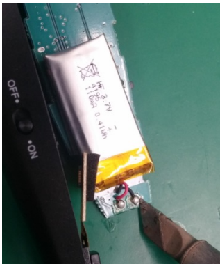
Remove battery wire.
