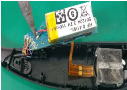
Remove battery wire.
