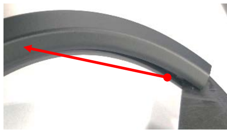
Insert the tool to the edge, and then disassemble from right to left.
