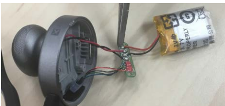
Remove battery wire.
