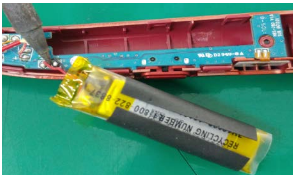
Remove battery wire.
