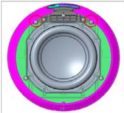
3) Disassemble of the Jersey Assy (2 screw)
