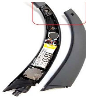
Insert the tool to the edge, and then disassemble from right to left.
