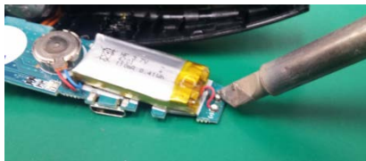
Remove battery wire.
