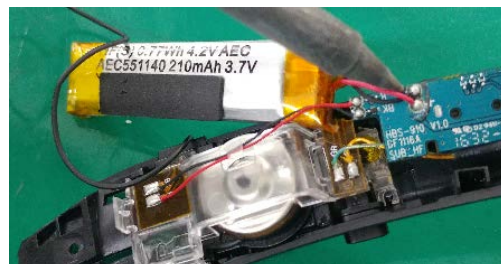
Remove battery wire.
