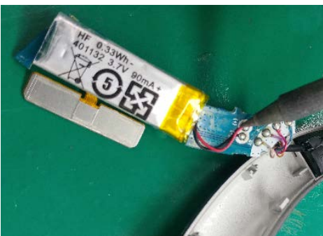
Remove battery wire.
