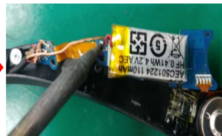
Remove battery wire.
