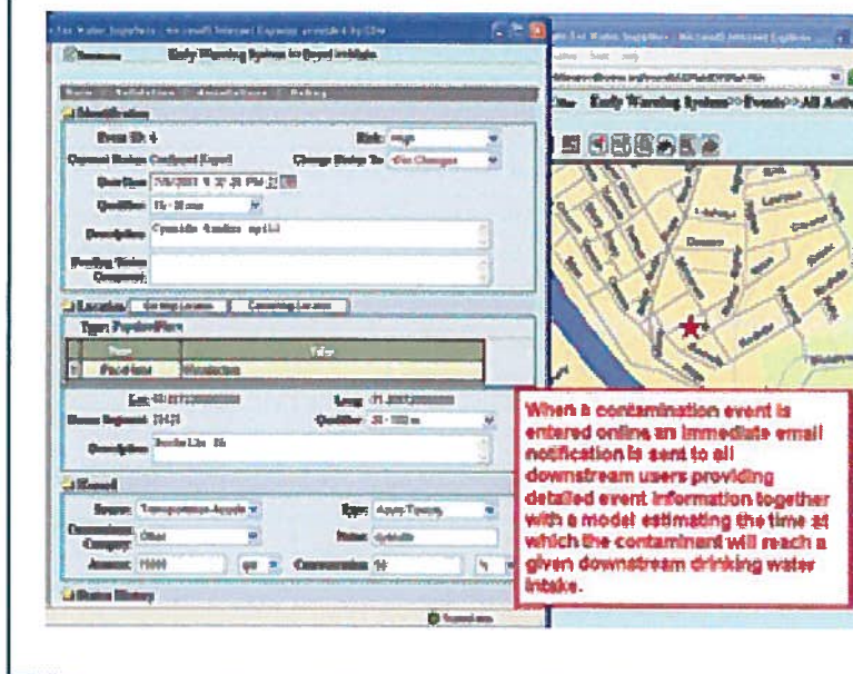
FIGURE 6 Sample Delaware Valley early warning system user interface screen for a hypothetical spill event—water quality event report form
