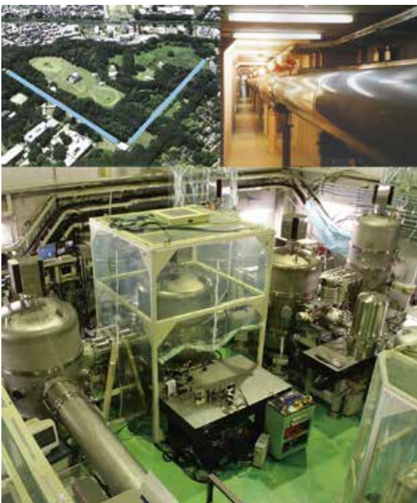
▲TAMA300, the world's first science grade Gravitational Wave Telescope, based on a laser interferometer now serves as a test-bed, developing new technologies for KAGRA. (Upper Left) Areal photo, blue shows locations of arm tunnels. (Upper Right) Inside an arm tunnel. (Bottom) Input/output optics lab.
