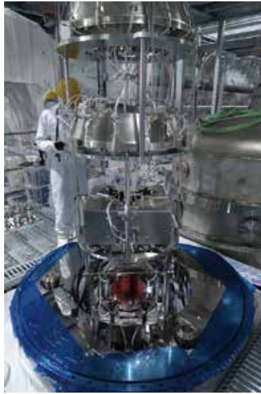
◀ The KAGRA beam splitter suspension system about to be installed into a vacuum chamber.
