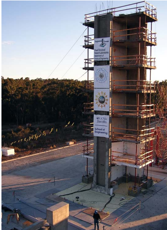
Large-scale seismic safety tests are completed with the full-scale seven-story concrete building constructed on the outdoor shake table at the Englekirk Structural Engineering Center (Photo credit: José I. Restrepo, Charles Lee Powell Structural Research Laboratories, University of California, San Diego).
