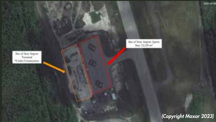
Figure 9: Imagery from March 2021 illustrates the newly constructed runway apron as well as the construction site for the new airport terminal. The size of the new airport apron is 15,129 m 2 , almost triple the size of the original apron (5,476 m 2 ).
