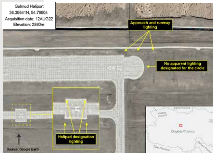
Figure 24: Golmud Heliport turning circle and lighting configuration
