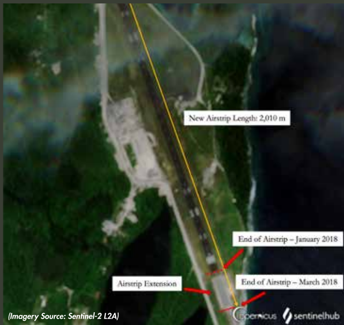
Figure 4: The Momote Airport's airstrip measured 2,010 meters in length on March 23, 2018.
