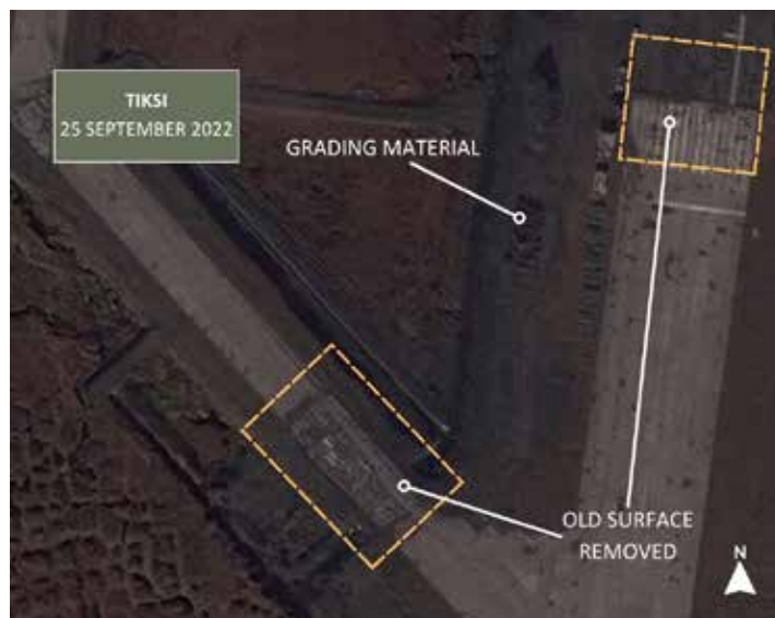
Figure 86: Tiksi taxiway repairs Copyright MAXAR 09/25/2022
