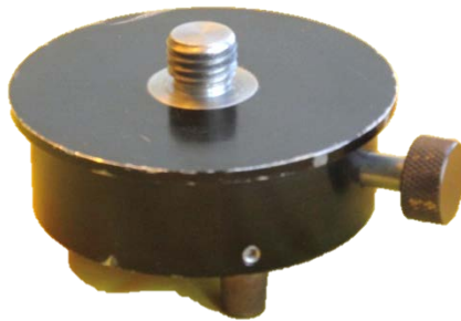
Figure 17: Top of tribrach adapter used for setup’s vertical point of reference
