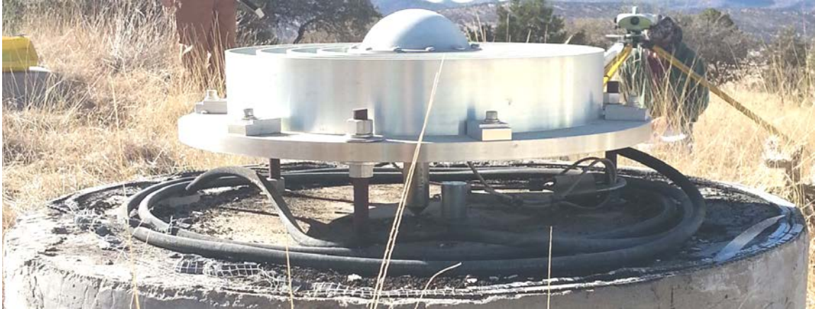
Figure 24: AOA GPS choke ring antenna plumbed over MCDONALD CORS MONUMENT (MDO1). Pictured with radome removed for survey observations.
