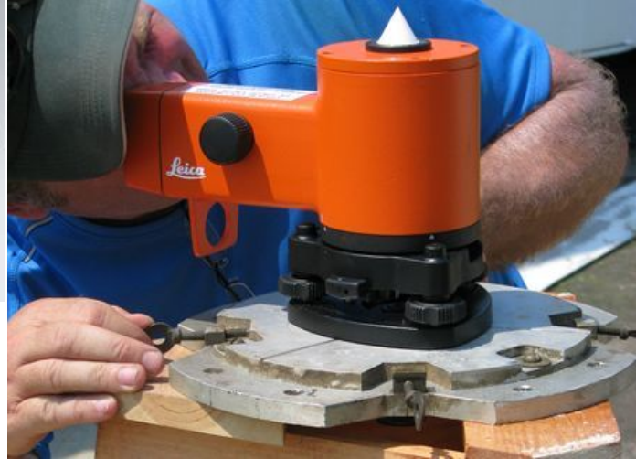
Figure 15: NL Collimator used to center the tribrach
