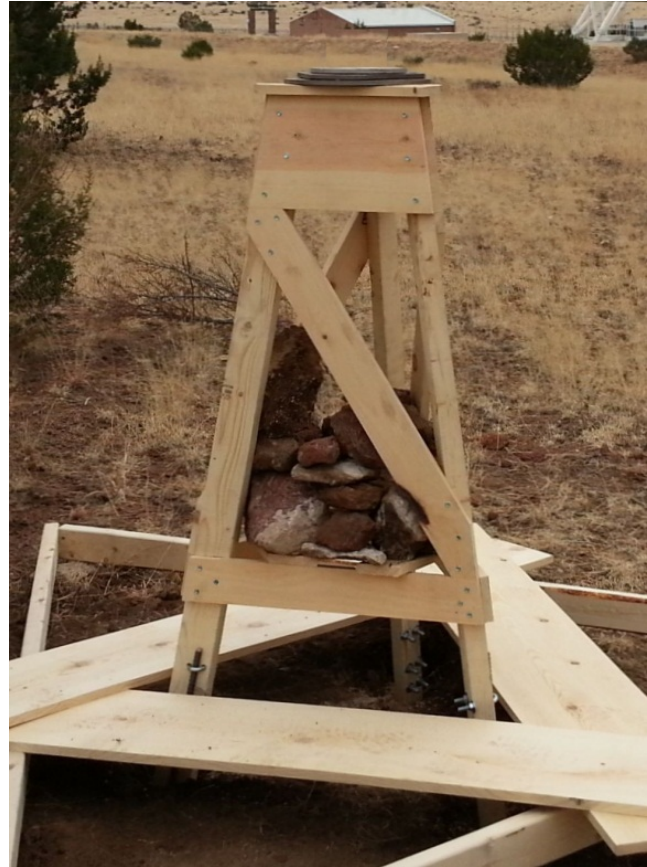
Figure 12: Typical U.S. Coast and Geodetic Survey wooden stand built over FT DAVIS VLBA RM 2. The three-legged stand is anchored solidly into the ground. The stones are “extra.” The stand is surrounded by a completely detached observer’s platform.
