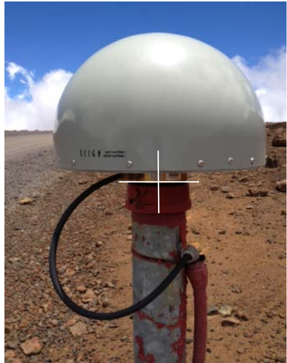
Figure 4 – SGT MKEA, the IRM associated with SGT MKEA is coincident with the ARP.
