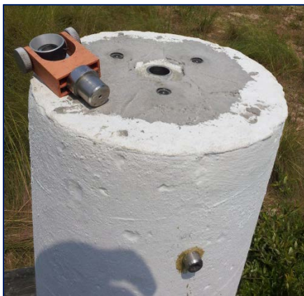
Figure 5 - CAL PIER A with NGS LR calibration reflector not installed. Cup embedded into top of pier is shown surrounded by three newly installed threaded inserts for attaching the survey team's translation plate and tribrach (Figure 7).
