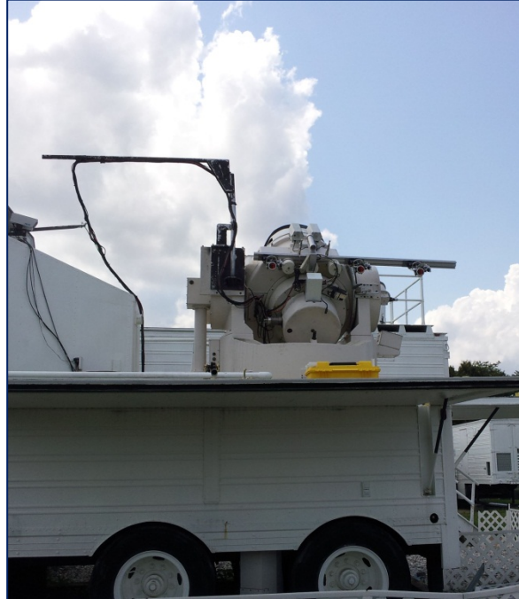
Figure 13. MOBLAS-7 with target bar mounted horizontally. Targets were positioned as they scribed circles about the horizontal (elevation) axis.
