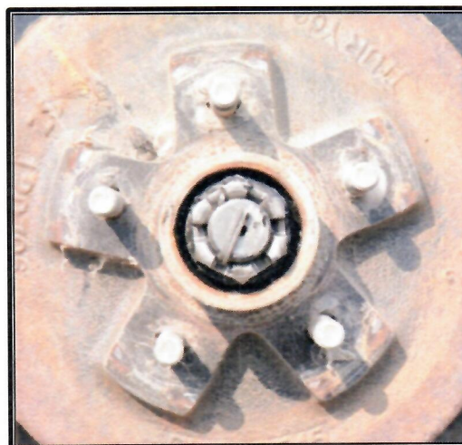
Left-Rear Spindle with Dust Cap Removed
