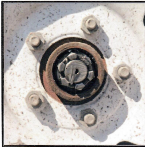
Left-Front Spindle with Dust Cap Removed
