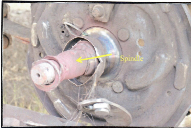
Damaged Right-Front Spindle
