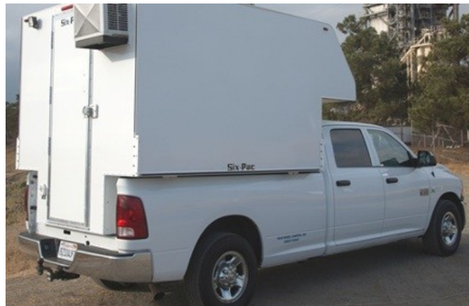
Figure H-2 Secured radiography darkroom truck
