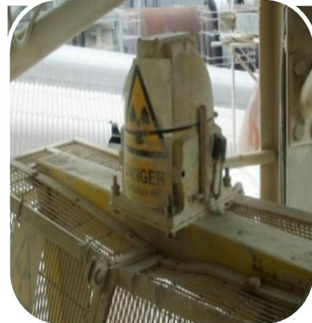
Figure D-1 Example of a fixed gauge
