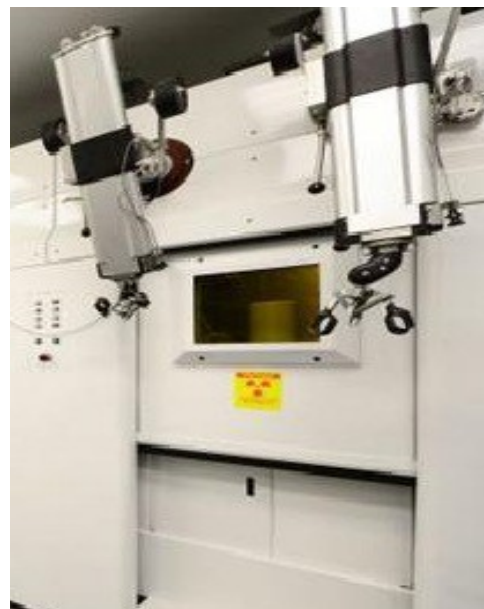
Figure F-1 Example of a hot cell with remote manipulators
