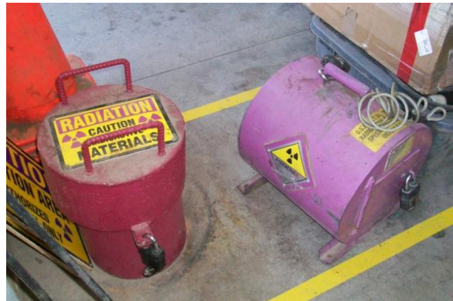
Figure G-1 Well logging source transport containers
