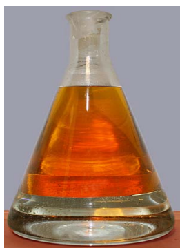
Green gasoline sits above water in this flask. Credit: Virent Energy Systems, Inc.
