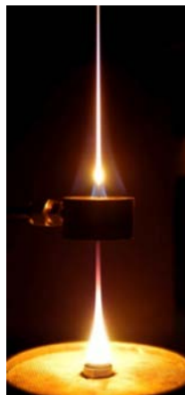
Soot oxidation will be studied in the yellow flame at the top of the ternary flame system seen in this image. Credit: Haiqing Guo and Peter B. Sunderland, University of Maryland, College Park.
