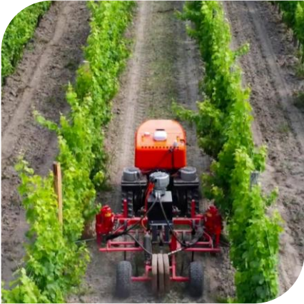
Robotized Mechanical weeding for vineyard
