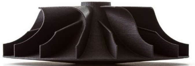
Be wary of warpage, as seen in this MJF example. The thinner a part is and the closer it is overall to the minimum feature size, the more likely it is to warp.
