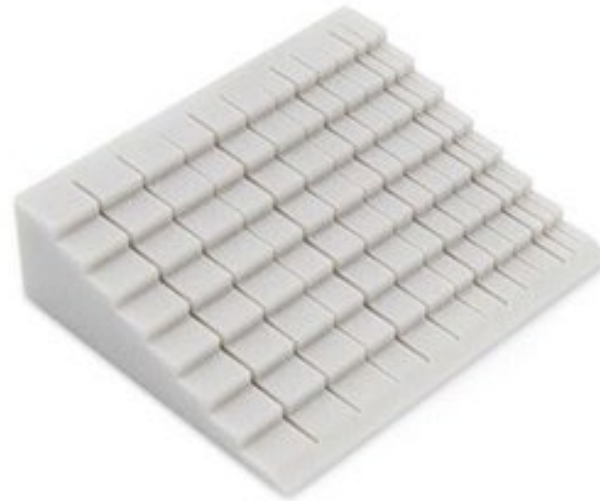
Channels dimensioned below 0.030 in. had a difficult time forming this PA12 40% glass-filled part.
