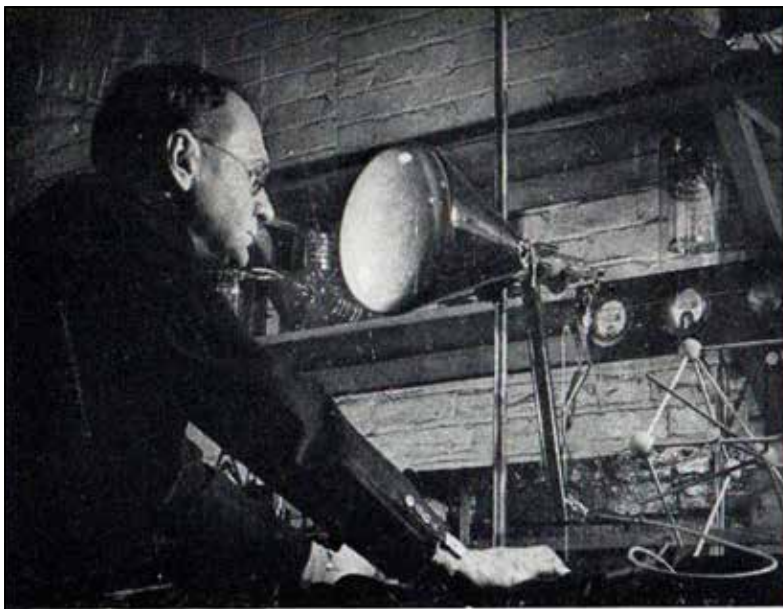
Testing the Kinescope, heart of the television receiver, in the RCA Research Laboratories.
