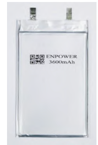
Mass-energy density 520Wh/kg class battery jointly developed by SoftBank and Empower Greentech
