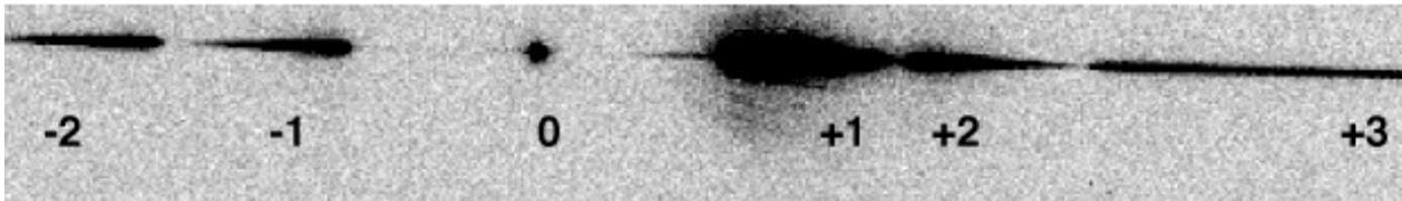
Figure 6.17: Fully dispersed spectrum for white dwarf GD153 with WFC/G800L. The numbers indicate the different grism orders.
