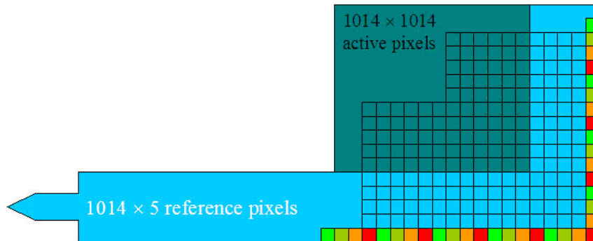
Figure 5.18: Schematic layout of the active pixels (dark shading) and of the reference pixels at a corner of the WFC3/IR detector. The color coding represents different values of the reference pixel capacitance.
