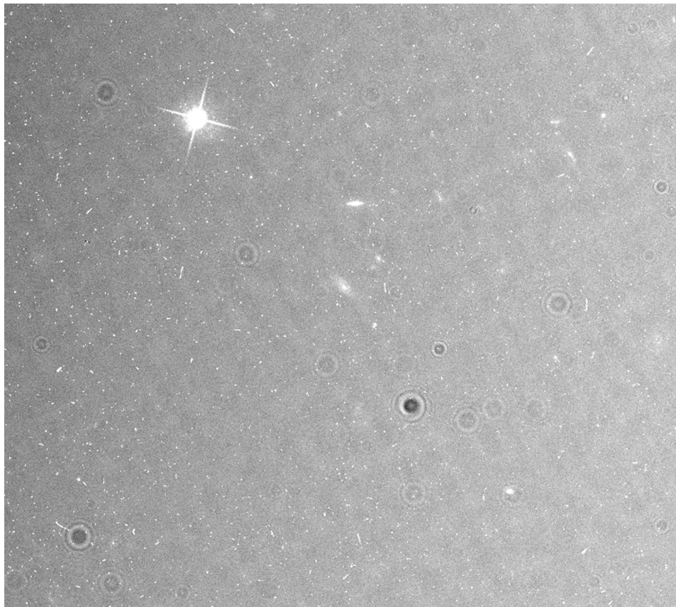
Figure 4.5a Close-up of dust rings in HST_9468_a8_ACS_WFC_F814W_drz.fits. In this example, the target declination was 62^\circ . At the time of the exposure, the sun altitude was -2^\circ , just below the Earth horizon. Although the observation was executed while the telescope was in Earth shadow, some sunlight, scattered by the Earth's atmosphere, was able to illuminate the camera, casting deep shadows of dust particles on the CCD windows and filters.
