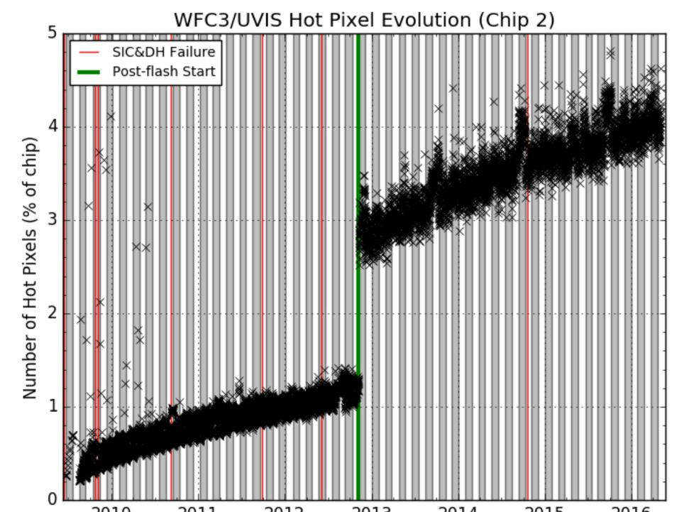
The median dark current (left) and number of hot pixels (right) over time for Chip 2 (Amps C & D). Dark current increases roughly 0.5 e-/hr/year and is currently ~8 e-/hr. Approximately 1000 new hot pixels above the 54 e-/hr threshold appear every day, currently occupying ~4% of each chip. Each month, the UVIS detector is warmed to +20C (shaded in gray/white regions), erasing 10-20% of the hot pixels.
