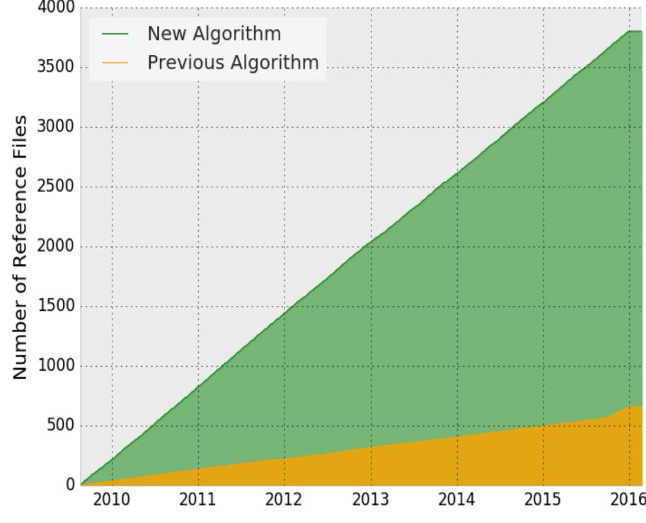
The cumulative number of dark reference files delivered to the Calibration Reference Data System (CRDS) from the start of Cycle 17 through the installation of CALWF3 v3.3 (02/23/2016) for (orange, 656 total). Observers with science data taken prior to the release of CALWF3 v3.3 may request their data through the Mikulski Archive for Space Telescopes (MAST) to obtain the improved products.
