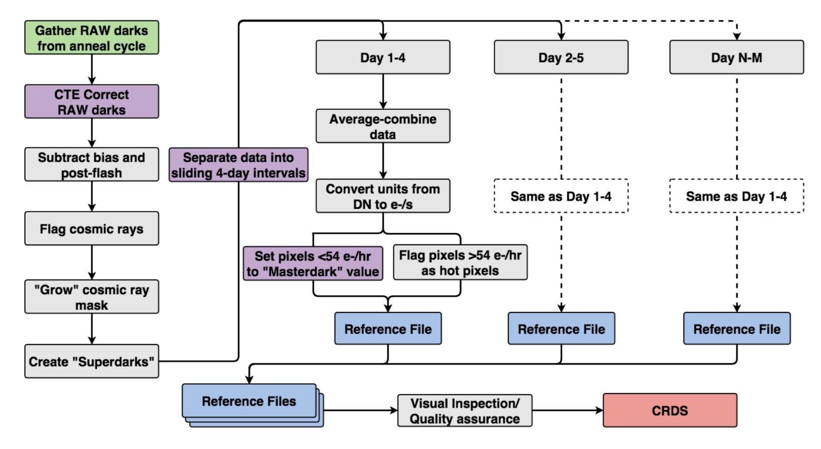
A new UVIS dark calibration algorithm (shown above) has been implemented in the release of CALWF3 v3.3. This update introduces several improvements (colored in magenta), which include:
