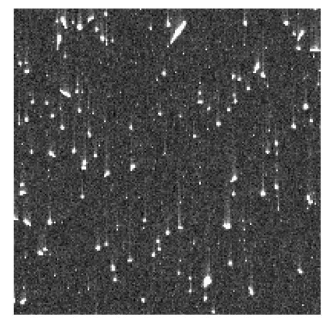
(Left) A 50x50 pixel region taken from a 900-second UVIS dark, showing the nominal features of background dark current, cosmic rays, and hot pixels (defined as pixels with dark current exceeding 54 e-/hr).
