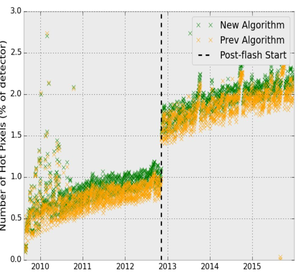
The number of hot pixels present in dark reference files over time for darks generated from the previous reference files generated from the new algorithm algorithm (orange) and from the new algorithm (green). (green, 3800 total) and from the previous algorithm The CTE correction allows for the detection of hot pixels that otherwise would have been immeasurable due to CTE losses.
