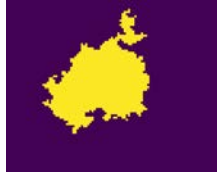
Figure 25 – The region of connected pixels that have a total number of pixels (area) greater than the input parameter.
