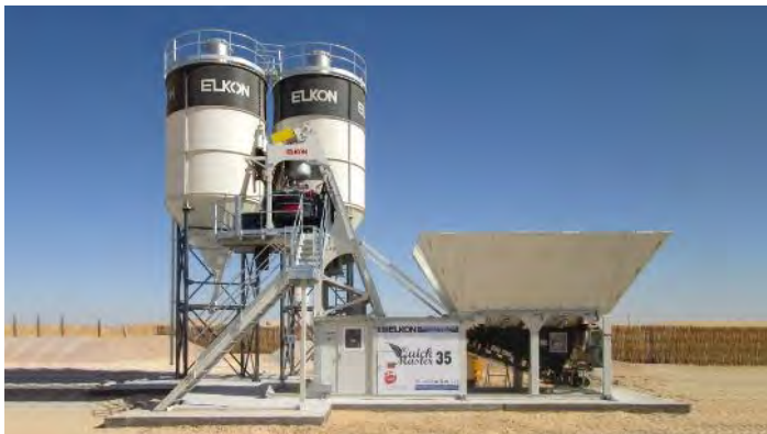
Example of a portable shotcrete batch plant that could be located in a staging area and used for canal lining.
