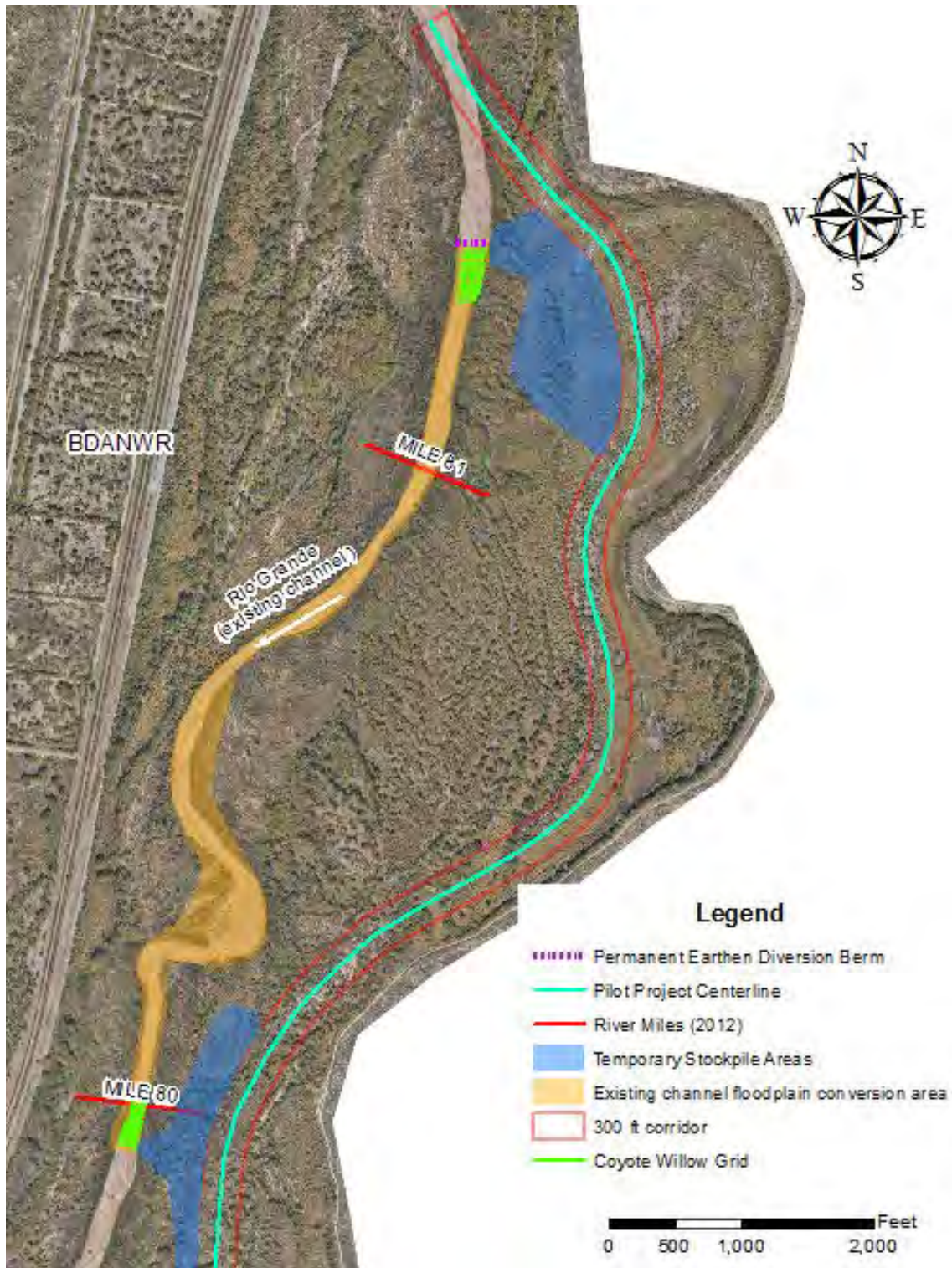
Figure 6: BDA pilot project centerline and 300 vegetation clearing corridor with existing channel floodplain conversion area and a view of coyote willow grids as part of the channel fill with vegetation stabilization. Coyote willow grids are shown at the upstream and downstream end of existing channel floodplain conversion area. The background imagery is the 2016 aerial photography (Reclamation).
