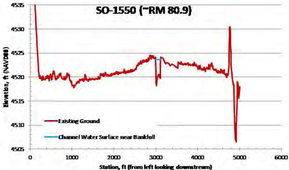
Figure 14: Example cross section (looking downstream) showing perched channel geometry in the proposed project area. Note that when the channel water surface elevation rises above the top of banks, flow will spill out and travel to low elevation areas in the floodplain.
