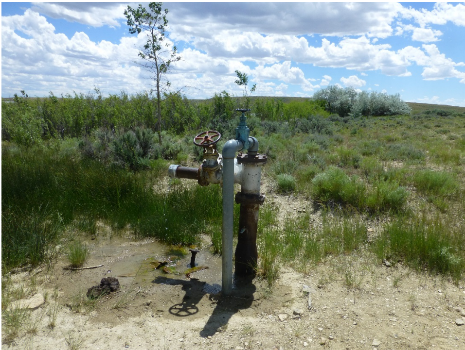
Figure D-6. Artesian well on the west side of Big Sandy Reservoir.
