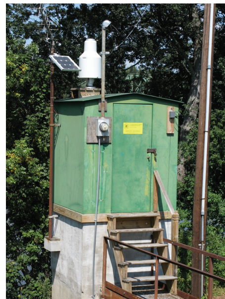
The Middle Atlantic River Forecast Center uses data from USGS stream gages to forecast river stages and flows in the Middle Atlantic Region. USGS field personnel are deployed to stream gage stations during periods of high water to compare stages with flows and help update and improve the Rating Curve.
