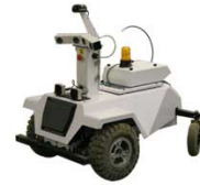
Figure 1. The robot weighs 70kg, measures 1 meter high, and can reach a maximum speed of 1.3 meters/second.
