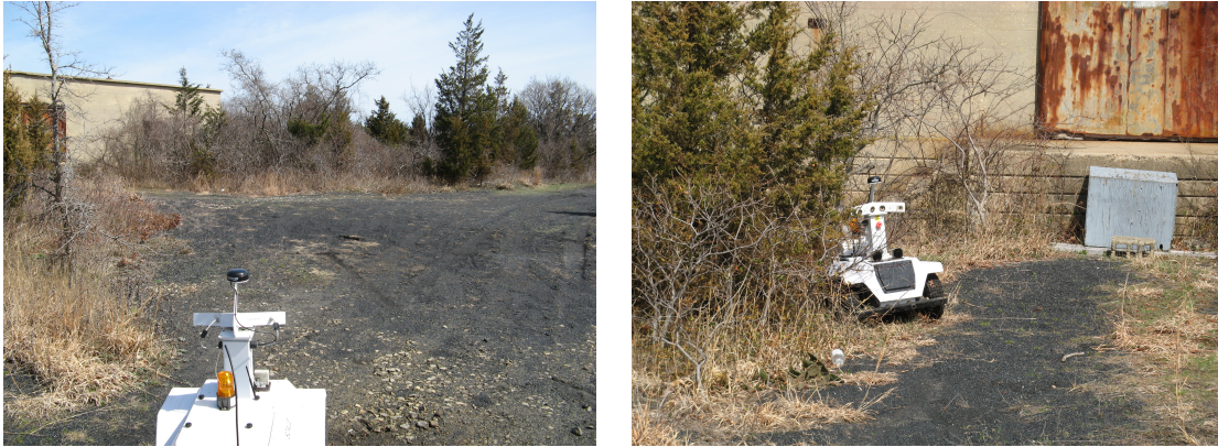
Figure 4. The testing site. Left : the robot is at the start point, facing the goal, which is 100m away, beyond the trees. The left path is blocked by a large building. The right path is clear. Right : the robot is stuck in brush when it runs without FAR-OD to guide it away from the dead end.
