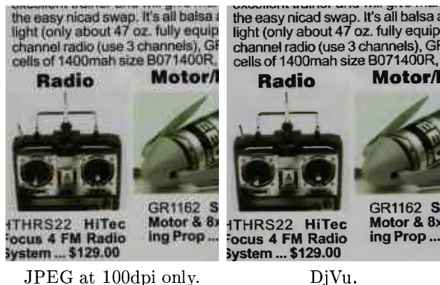
Figure 4: Comparison of JPEG at 100dpi (left) with quality factor 30% and DjVu (right). The images are cropped from hobby002 . The file sizes are 82K for JPEG and 67K for DjVu
