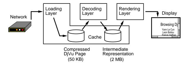
**Figure 1.** The three layers of the DjVu viewer: the loading layer loads and caches document components, the decoding layer constructs the intermediate representations, and the rendering layer computes the image pixels.
