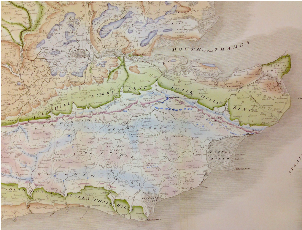
Fig. 1. Part of Smith's (1815) map for SE England. It shows the geological units in colour, hand-painted on a monochrome printed base map created by the cartographer John Cary. This shows principal settlements, major roads and rivers.
