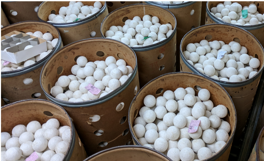
Figure 32: Rounds prepped for stitching cover.
