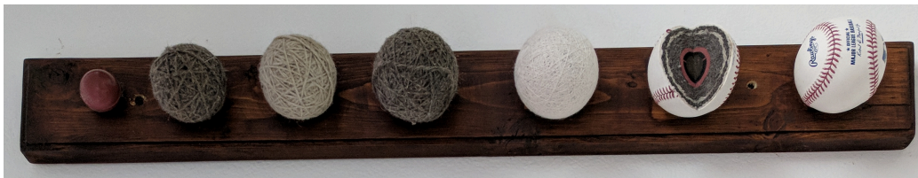
Figure 29: Cross sections of the components comprising the MLB baseball.
