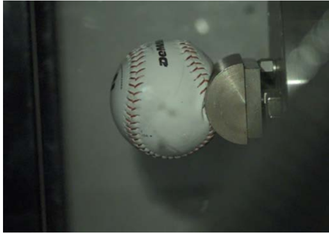
Figure 41: Image of a softball impacting a rigid cylinder to measure its cylindrical coefficient of restitution or CCOR.
