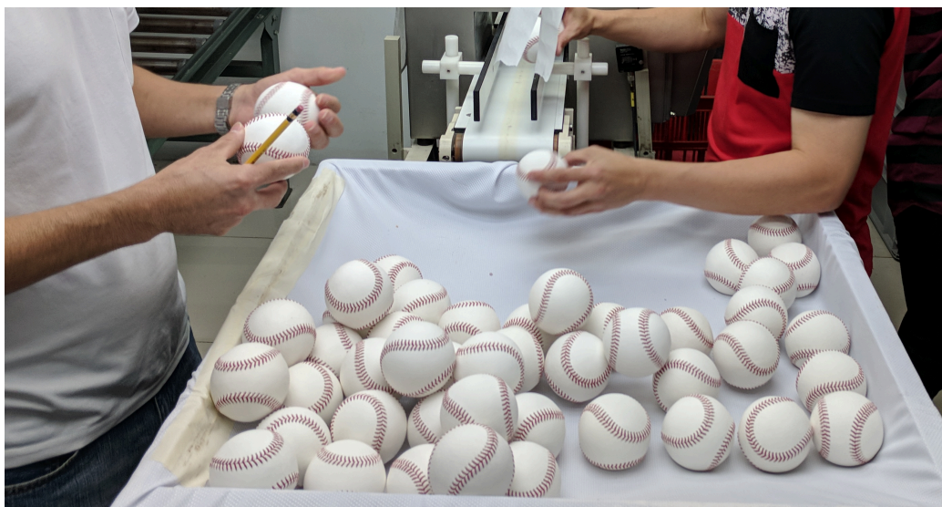
Figure 37: Ball inspection after stitching.
