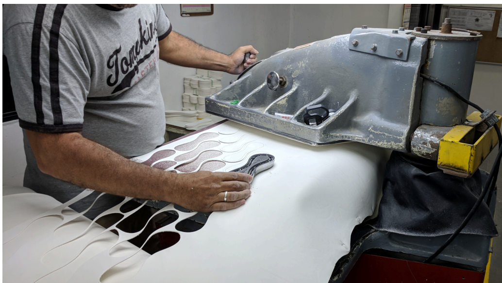
Figure 33: Cutting of leather panels.
