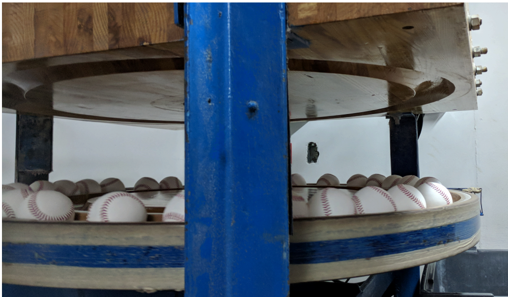
Figure 36: Ball rolling to flatten seam.
