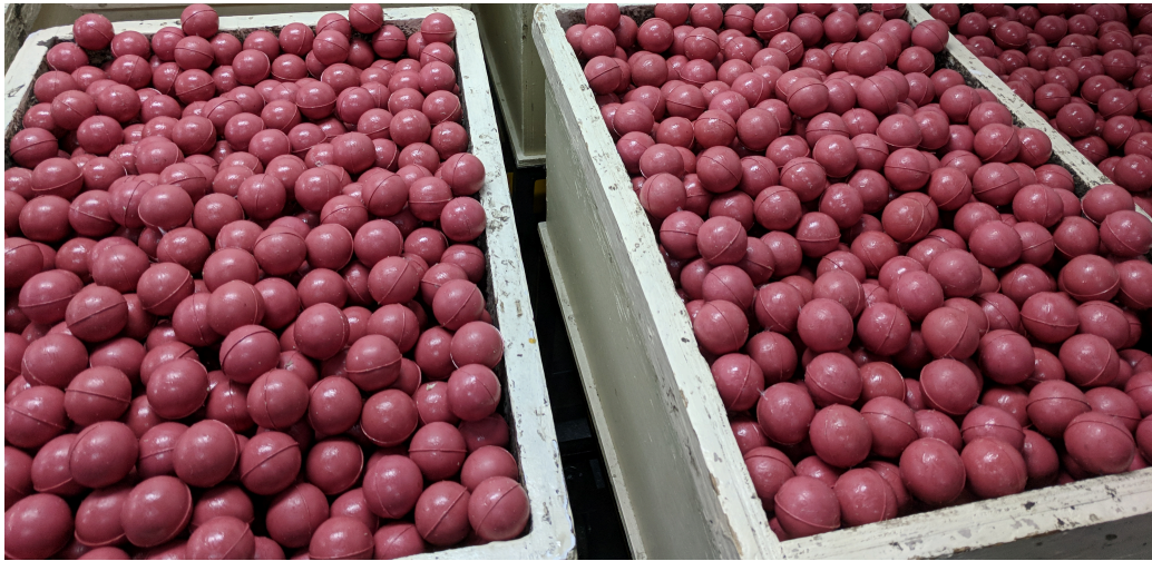
Figure 30: Pills prepped for winding.
