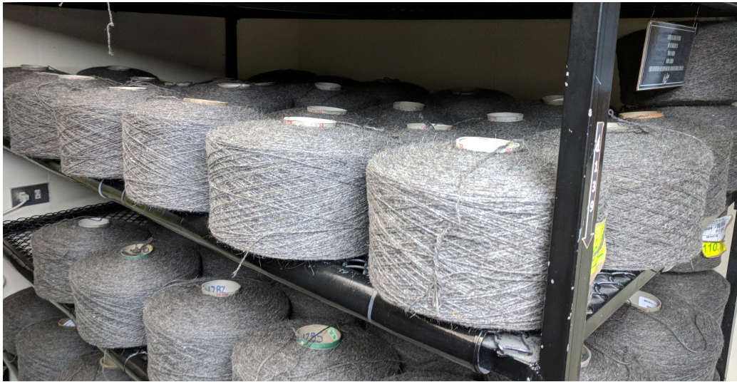
Figure 31: Wool in conditioning prior to winding.
