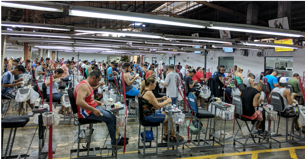
Figure 35: Manual sewing of leather covers.
