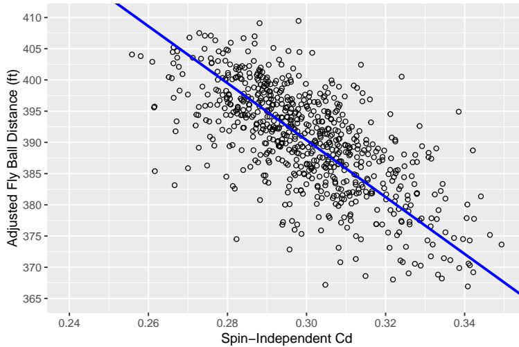
Figure 10: Relationship between fly ball distances and the spin-independent drag coefficient. The distances are for 100 mph exit velocities and launch angles 25^\circ - 30^\circ and have been controlled for air density, spin rate, and spin axis. The plot shows that the adjusted distances are inversely proportional to the spin-independent part of the drag coefficient, as expected. The total spread in distances, \sim 8 ft rms, is due primarily to the ball-to-ball variation in C_d ( \sim 6 ft), with the remainder due to experimental noise.
