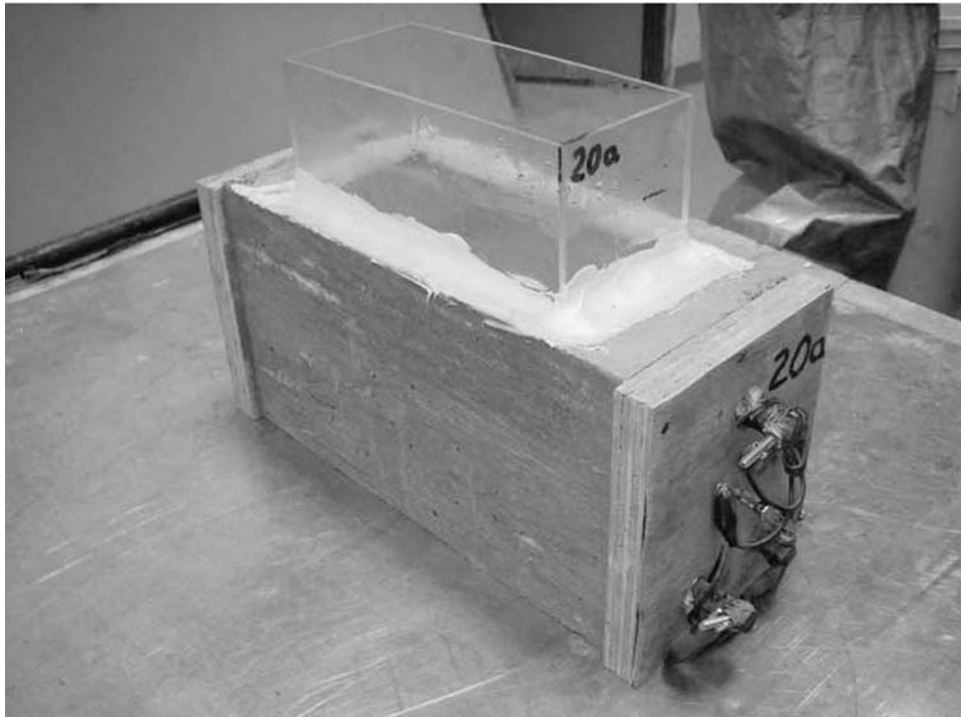
Figure 10-1. ASTM G 109 specimen illustration.
