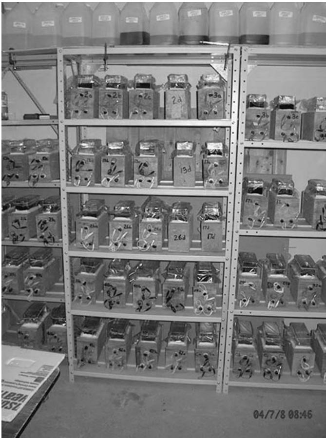
Figure 10-2. ASTM G 109 specimen setup.
