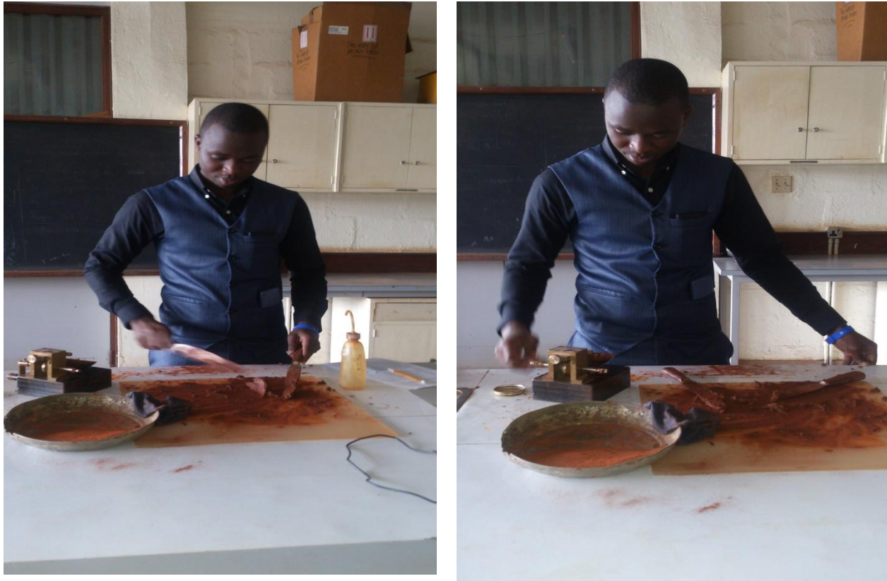
Figure 22: Plastic limit by casagrande method
