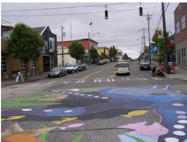
A painted intersection at 6th Ave and Pine St. expresses neighborhood character while also serving as a traffic-calming device.
