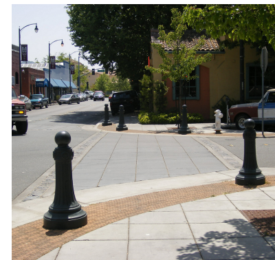
Curb extensions, bollards, and special pavement treatments contribute to a safe and comfortable intersection for pedestrians.
