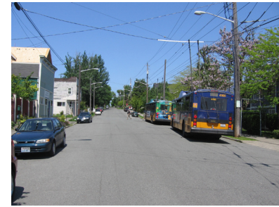
A wider roadway width is required for residential streets that are transit routes.
