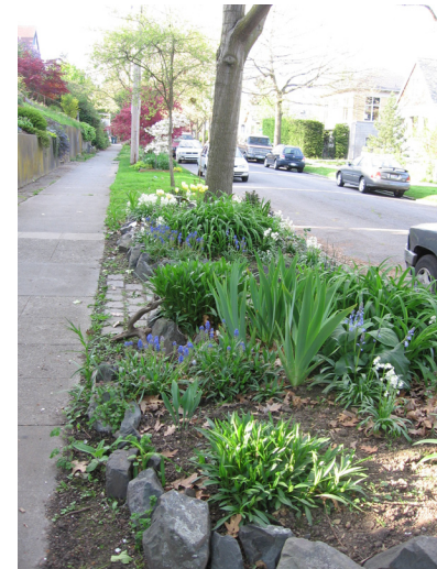
Planting strips that are a minimum 6 feet in width accommodate healthy tree growth and provide opportunities for additional landscaping.
