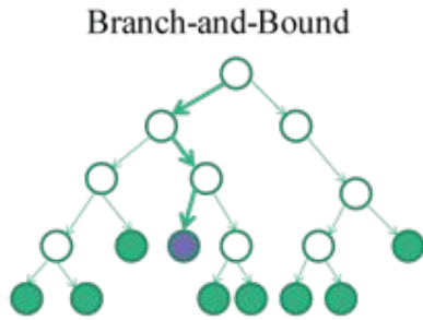
Figure 13: Each node of the branch-and-bound algorithm is a new IP problem.
