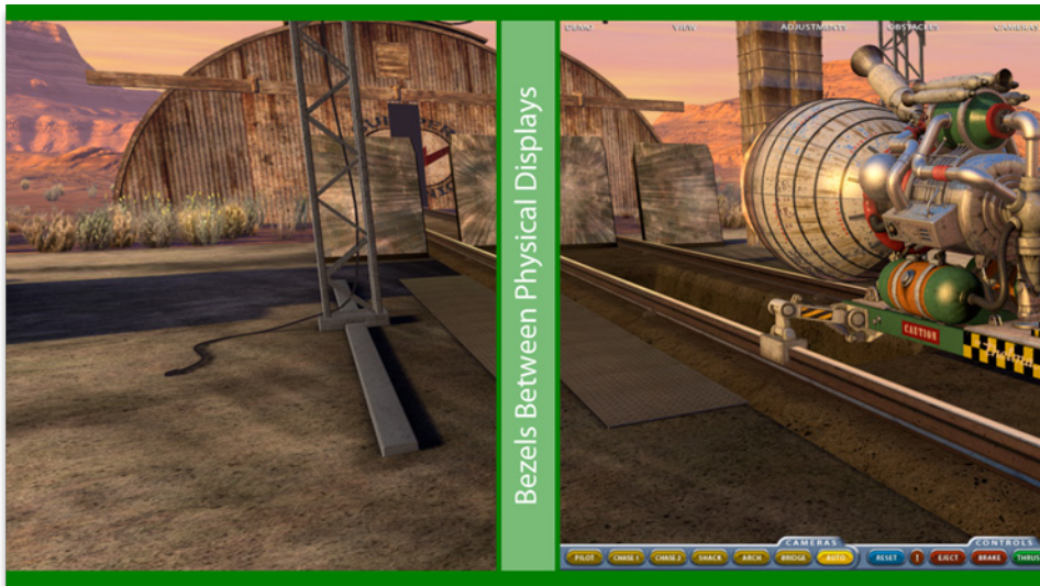
Figure 10. Lack of Bezel-Corrected Mode Shows Split/Elongated View Between Left and Center Surround Displays
