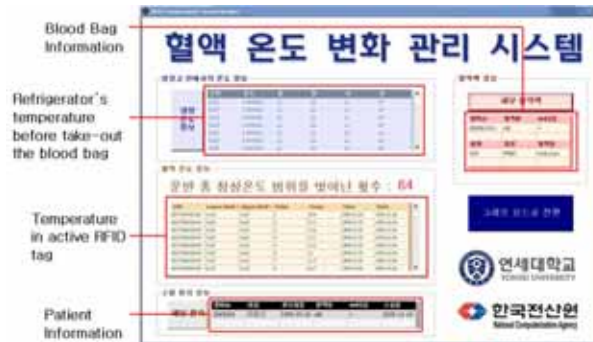
Fig. 7. Management system reporting the variation in temperature of the blood bag before a transfusion
