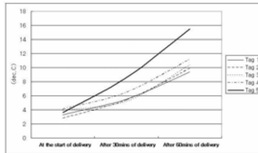
Fig. 9. Changes in temperature of the blood bags after removing them from the refrigerator
