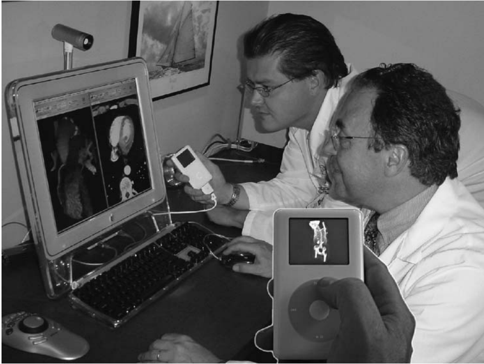
Image 1. Dr. Osman Ratib, on the front right, and Dr. Antoine Rosset, on the left back, using their iPod to quickly load and display DICOM images on the OsiriX software. DICOM images are directly loaded from the iPod without the need to copy them on the computer hard disk. The iPod is connected through the FireWire interface and is automatically recognized by the OsiriX software (displayed on the screen) as a DICOM storage.
