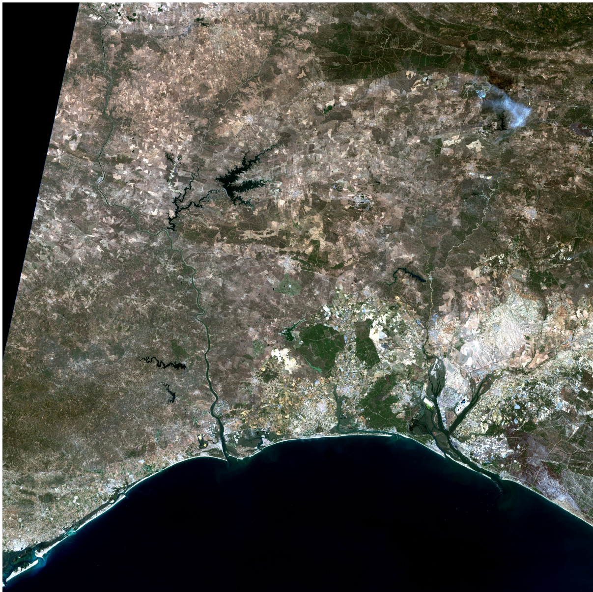
Figure 5. Result of applying radiometric corrections to the image and get radiation as if there was no Earth atmosphere (Bottom of the Atmosphere; BoA).
