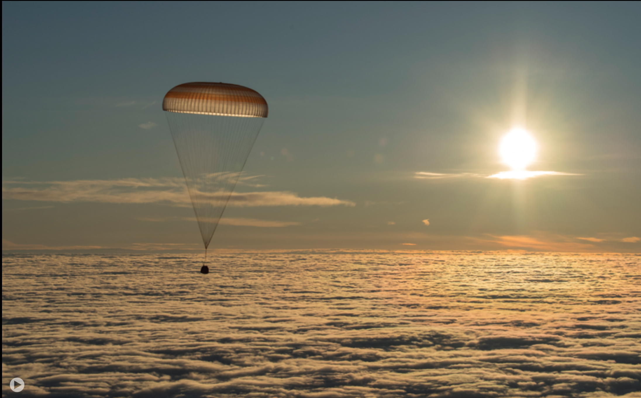
Three hours after leaving the Station, the Soyuz descent module deploys a series of parachutes to allow a stable descent at a speed of around 7 m/s (NASA)
