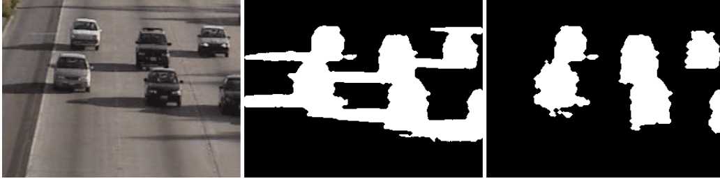
Figure 4.2: Input Image, together with Moving Object Detection Mask and Detection Mask after the Shadow Removal Algorithm Utilized
