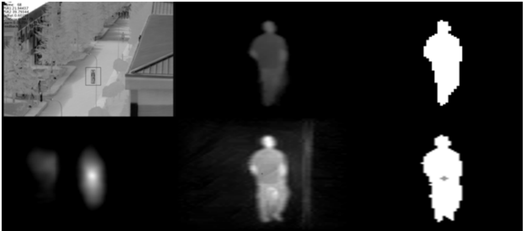
Figure 3.10: Updated and Current Saliency Maps with their Binarized Images at the Beginning of the Track
