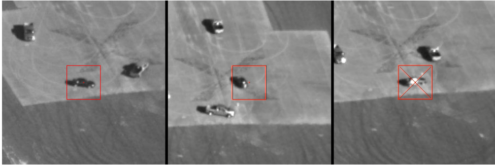
Figure 4.7: Illustrative Examples for Good Track (Left), Drifted Track (Middle), and Track Lost (Right)
