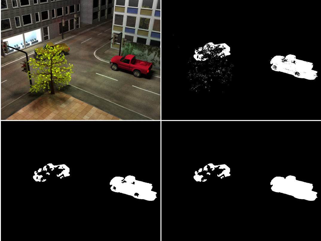
Figure 4.1: First Row: Input Image and the SAGMM Output; Second Row: Output of Median Filtering + Morphological Closing, and Output of Filling Process
