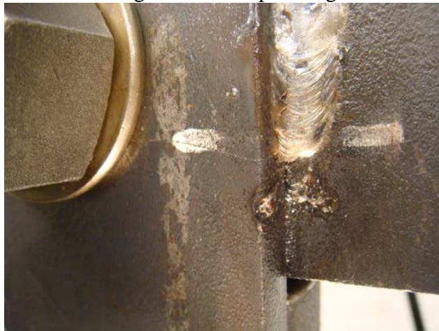
Figure C-12: Fatigue crack at front face lower right tack weld toe for specimen TW-3LN-12-3
