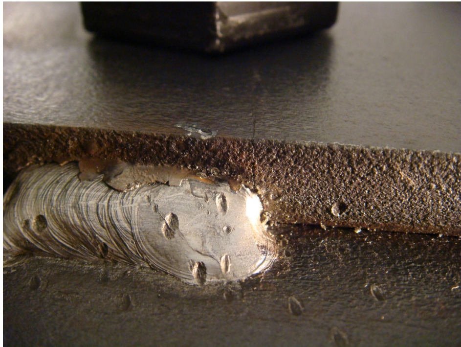
Fig C-15: Fatigue crack at tack weld toe for specimen TW-2LN-12-1
