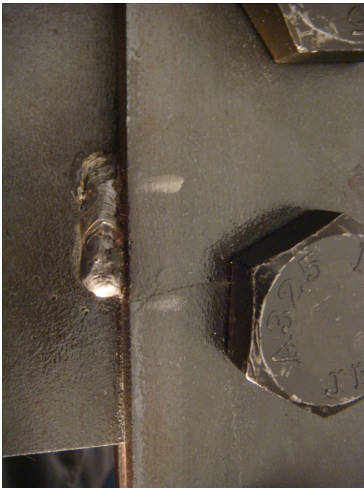
Fig C-21: Specimen TW-2LM-12-1 Crack
