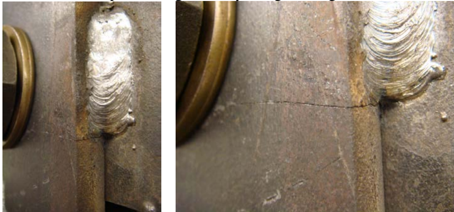
Fig C-4: Fatigue crack in lower right weld on front side of specimen spreading transversely into the splice plate
