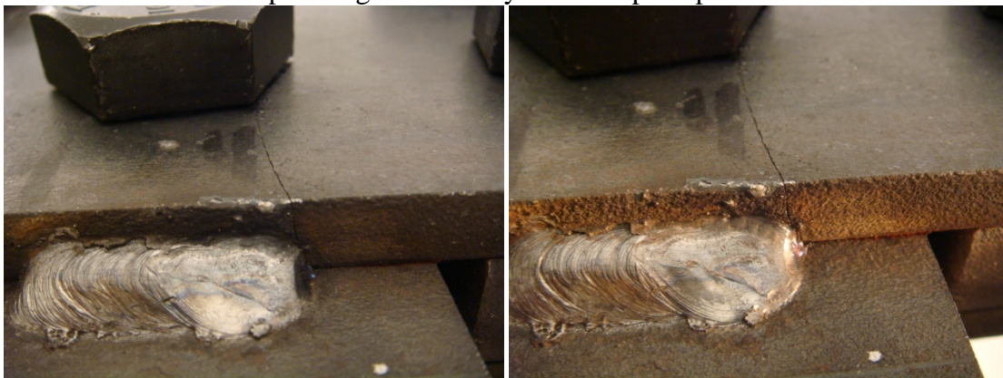
Fig C-5: Fatigue crack in lower left weld on back side of specimen spreading transversely into the splice plate
